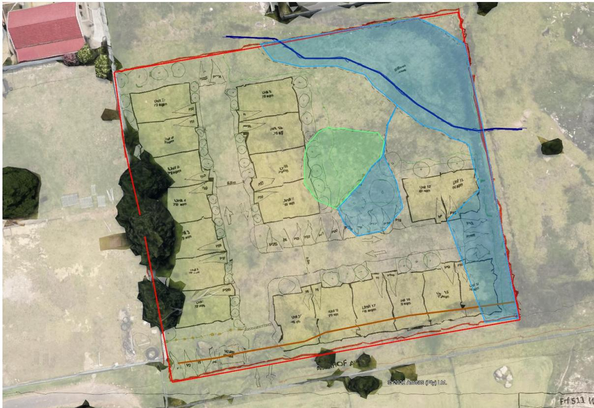
**Figure 2.** Final layout plan for the site, overlaid in Google Earth, together with the mapped wetlands within the site where the green polygon comprises of seasonal, grass dominated wetland and the blue polygons more permanently wet and bulrush dominated wetlands
