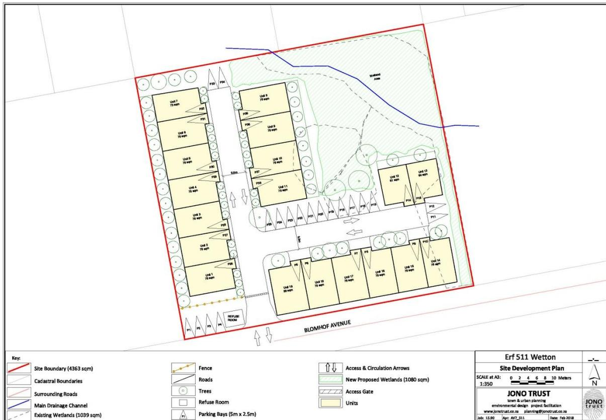
Figure 1. The proposed final layout for Erf 511, Wetton
