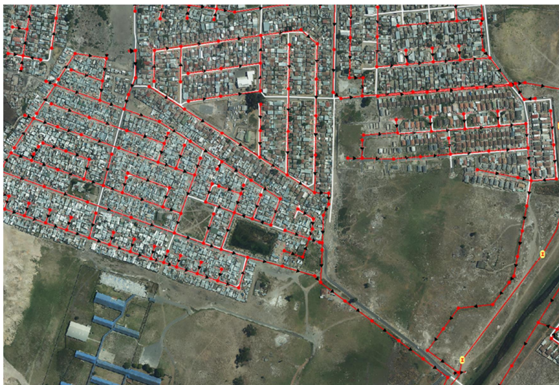
Figure 2-2: Existing Foul Sewer Network
