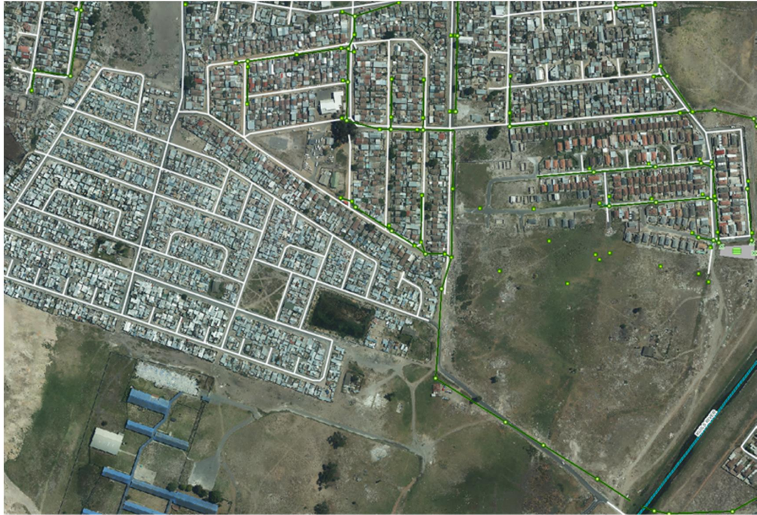
Figure 2-4: Existing Stormwater Network
